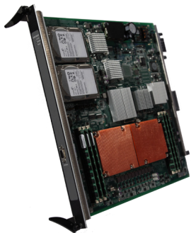
Crossbeam X-Series Application Processor Module (APM-9600) running McAfee Firewall Enterprise v8.1
