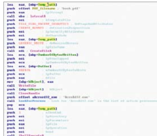
Figure 4: The malware looks for Acrobat Reader (AcroRd32.exe) and then opens the innocent file book.pdf .
