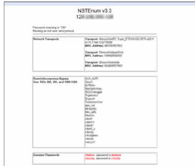
Figure 17. Two user accounts discovered using passwords that are the same as the username.
