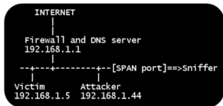
Figure 2. Man-in-the-middle attack exploiting WPAD.
