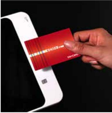
**Image 1.** Empathy's highly secure payment devices are available in rugged eight-inch and 10-inch tablets. Devices are equipped to read MSR cards, IC Cards, and include an NFC reader/writer, wireless LAN, wireless WAN, and Bluetooth capabilities.
