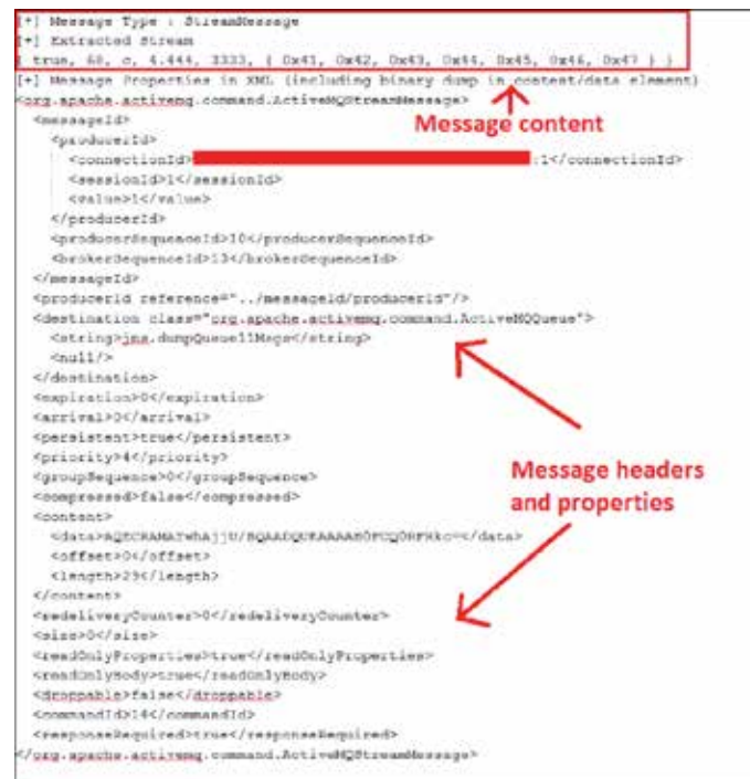
Figure 21. JMS destination's StreamMessage dump with JMSDigger.
